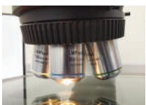
Infinity Long Working Distance Plan Achromatic Dark Field Metallurgical Objective Set (5x, 10x, 20x, 50x, 100x)
